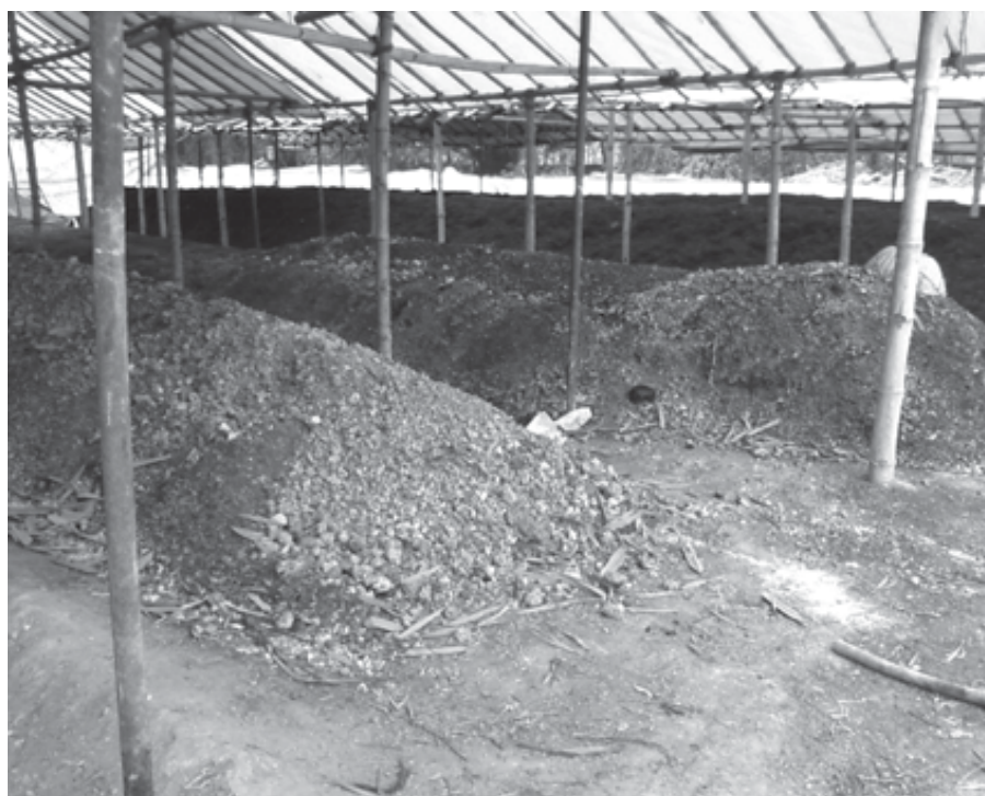
Effluent sludge with coir pith and Ayurvedic waste being processed as compost
